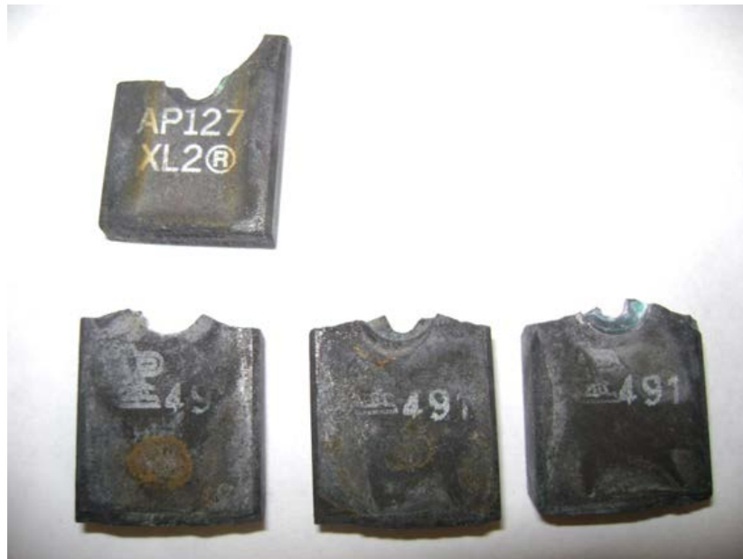
Figure 2. Brushes from CBP159's starter/generator
