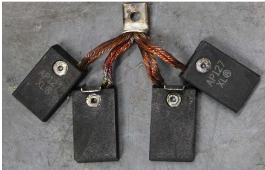
Figure 1. An intact single rivet brush assembly
