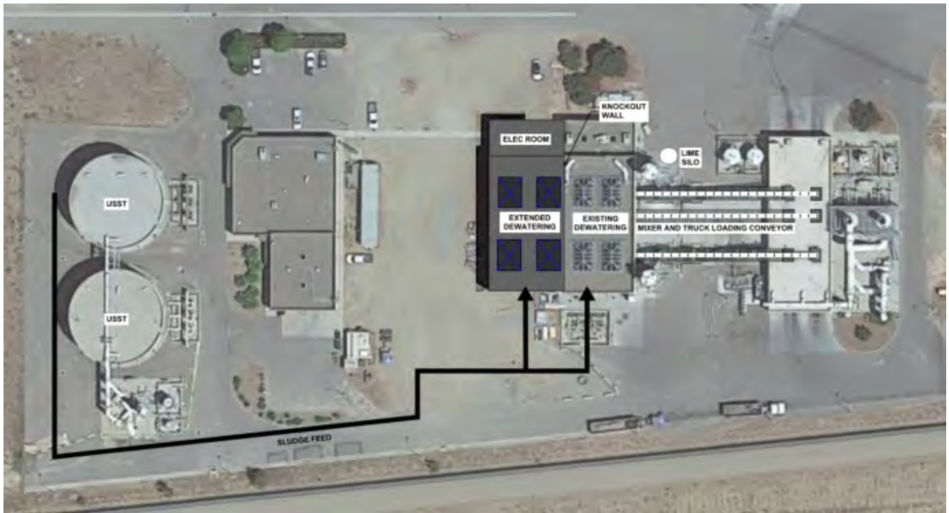
Figure 6-20. Dewatering Expansion to Add Third Train
