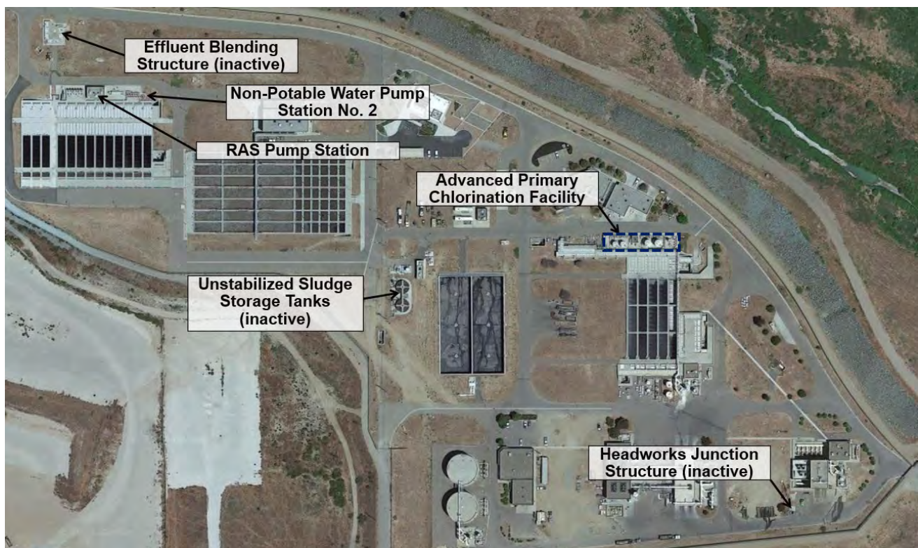
Figure 4-27. Advanced Primary Chlorination Facility and Dose Locations. Off-site Canyon Collector/Tank Drain Joint Structure not shown.
