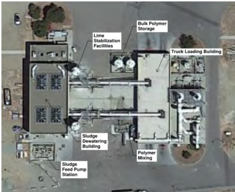
Figure 6-11. Solids Processing Location Plan
