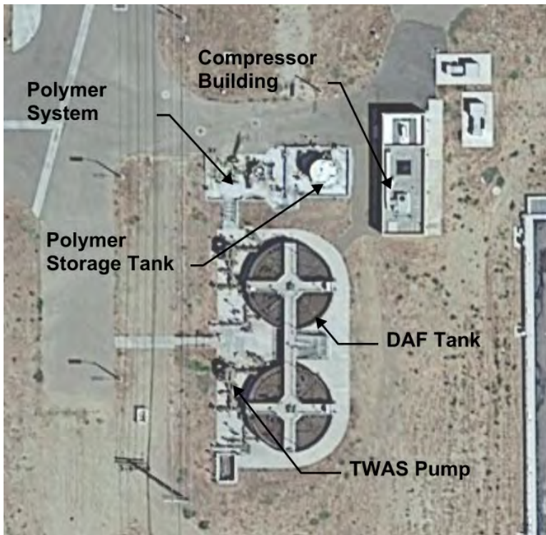
Figure 6-1. DAF Unit Existing Facility
