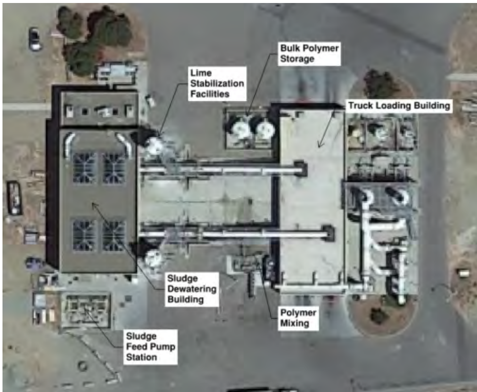
Figure 6-21. Solids Processing Location Plan
