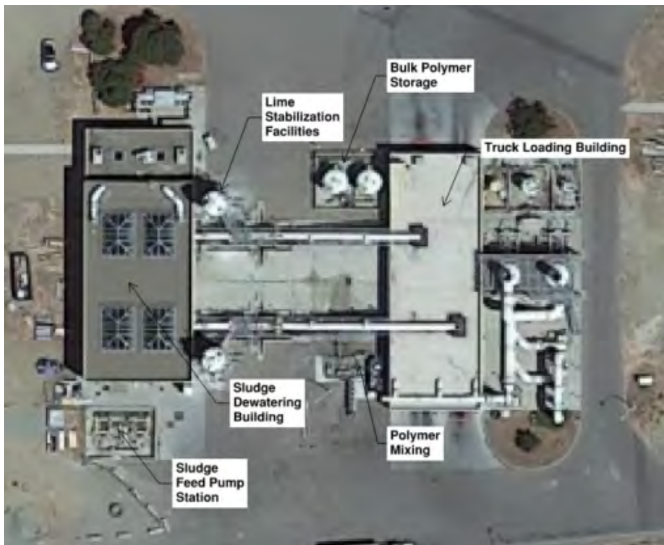
Figure 6-23. Solids Processing Location Plan
